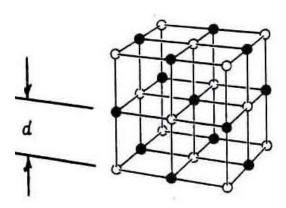
The first condition for Bragg "reflection" is that the angle of incidence  $\theta$  equals the reflection – this is as for optical reflection and infers that any detector of the reflected rays must move through an angle  $2\theta$ , the 2:1 spectrometer relationship. The second condition is that reflections from several layers must combine constructively:
