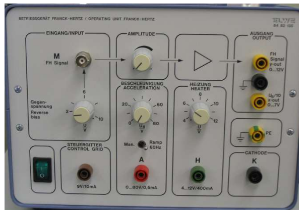
Figure 3. Franck-Hertz Control Unit
